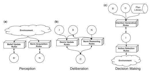
Fig. 1. Reasoning Phases in a Normative BDI Agent. The sets that contain the cognitive and normative elements (i.e. the sets B, D, I, N) are represented as circles. The reasoning processes are represented as boxes where: the input links represent the information used by the reasoning process, and the output links represent the information updated by the reasoning process.
