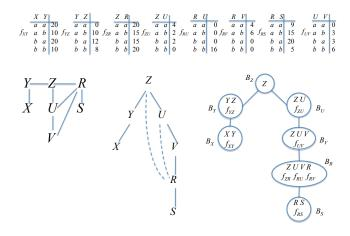
Figure 6: DCOP instance, each agent holds a variable, domains are  $\{a, b\}$ , cost functions are indicated. From left to right: constraint graph, DFS-tree rooted at Z, the corresponding bucket tree.
