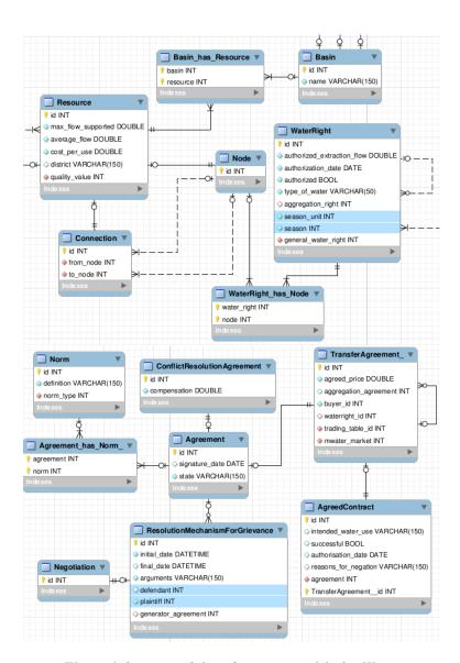
Fig. 5. A fragment of the information model of mWater
