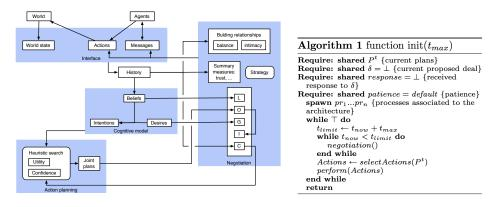
**Figure 1.** Agent architecture. White boxes represent data or concepts, boxes with round corners represent processes and arrows represent data flows.
