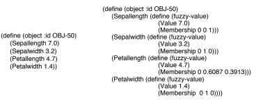
Fig. 2. On the left there is a propositional representation of an object. On the right there is the representation of the same object extended with the membership vector.
