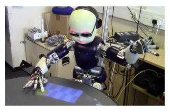
Fig. 1. iCub interacting with the virtual keyboard shown by the Reactable tactile interface. The finger is used to control the virtual object, which is used by our software to know which sound to play.
