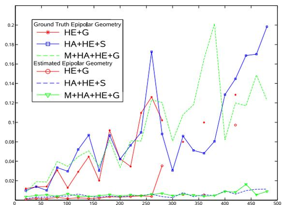
Figure 3: Mean distance error of a match to the estimated epipolar sinusoid and to the ground truth epipolar sinusoid.
