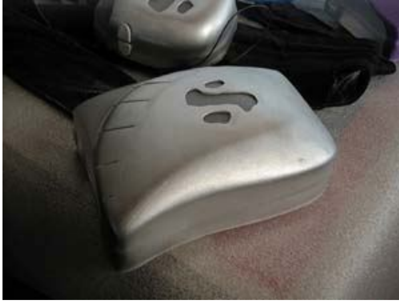
Fig. 2. The wearable computer also known as “the parrot”. The CPU is on the front unit while the back one hosts sensors and batteries.
