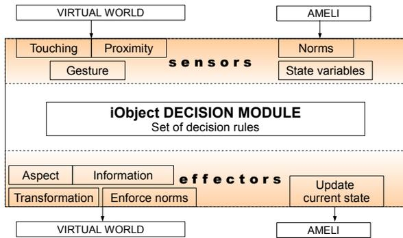
Figure 1. Structural components of an iObject
